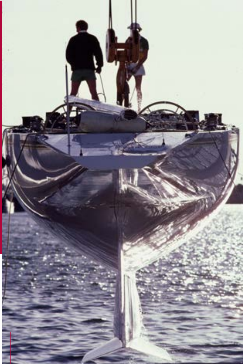
Digitisation of an image showing Australia II with the winged keel. Photo by Roger Garwood © WA Museum
