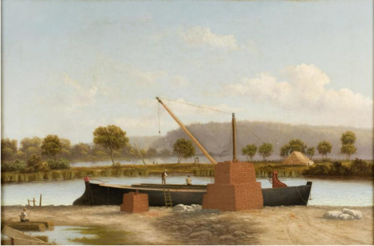
Figure 10. Swan River barge or flat shown in the oil painting 'Brick loading on the Swan River'. Note rudder, size of deck hatch coaming, crane derrick and mast, and windlass at bow. (Artist: Valentin Delawarr, Art Gallery of WA, 1975/0P17)
