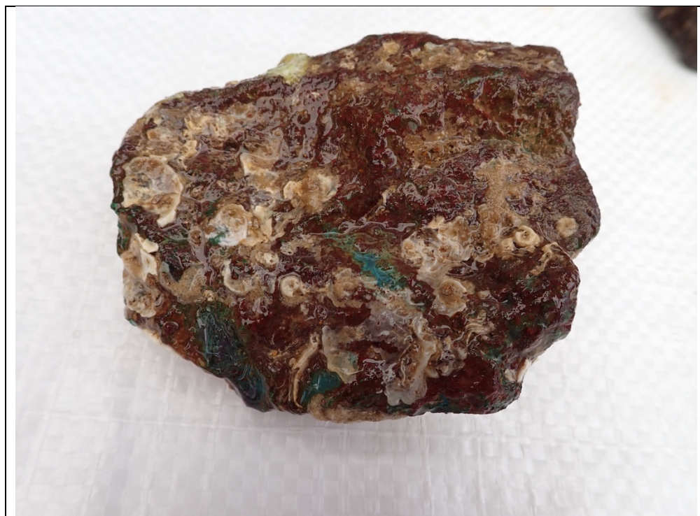
Figure 7 GLB-001 copper ore sample. Note green-coloured copper oxide visible. (WA Museum)
