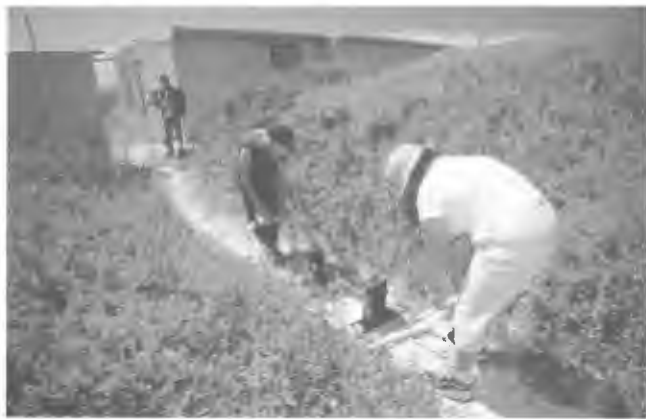
Figure 17. Adam O'Neill assisted by MAAWA volunteer, Holly Cassin, using the Pulse Echo 100 GPR to survey a path on Beacon Island.
