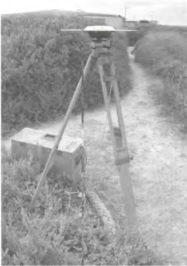
Figure 8. Trimble 4000 SSI Static GPS station setup on Beacon Island (BE1). The point is marked with a star picket and protected by a yellow cap when not in use.
