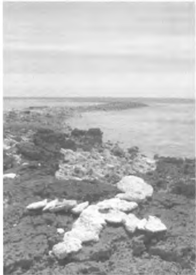
Figure 9. Example of a target cross—this particular one was placed on Hall Island. Note the black circle in the centre which will enable identification in the photograph accurate to a few centimetres.
