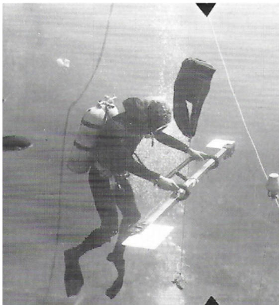
Figure 3: Underwater operation of the stereometric double camera (Höhle, 1971)
