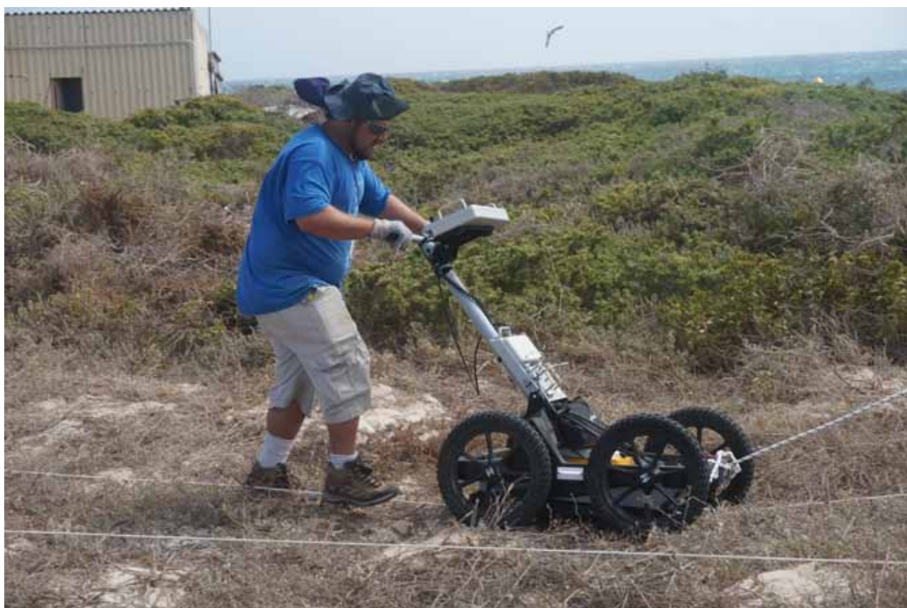
Figure 6. Jeff Shragge operating the 250 MHz GPR.
