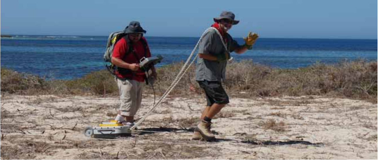
Figure 7. Jeff Shragge (left) recording and David Lumley pulling the 500 MHz GPR.
