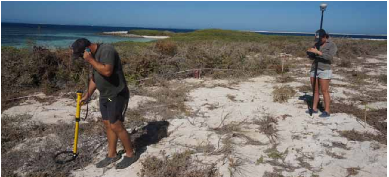
Figure 4. Metal detecting, Nic Bigourdan operating the ELSEC metal detector and Maddy McAllister operating the differential GPS system.
