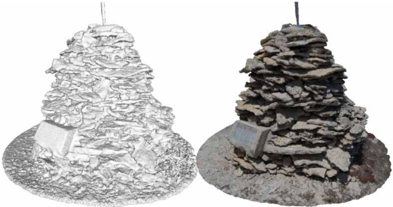
Figure 27. Reconstruction examples of the cairn, mesh on the left, textured mesh on the right.
