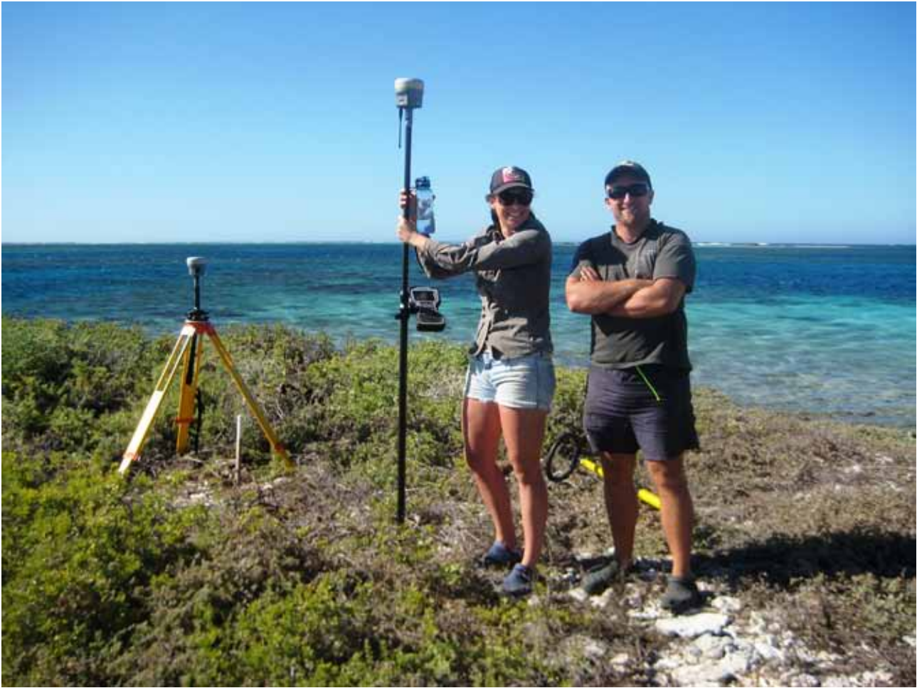
Figure 13. Maddy McAllister and Nic Bigourdan with the DGPS rover (pole) and the GPS base station (yellow tripod) in background.
