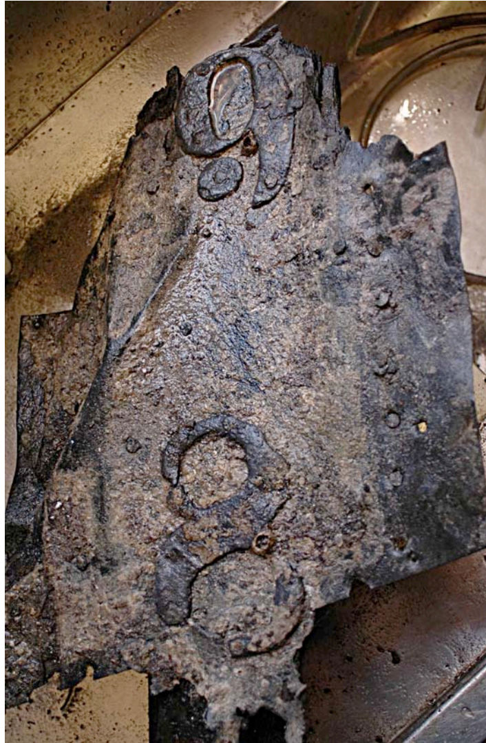
Figure 49. Stem post sheathing with waterline markings '8' and '9' feet (Jon Carpenter/ WA Museum).
