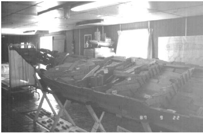
Figure 42. View of the model of the Shinan Ship showing the bulkhead arrangements.
