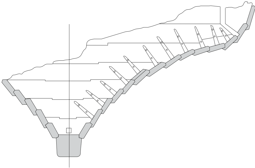
Figure 49. Shinan Ship cross-section of the Shinan Ship.
