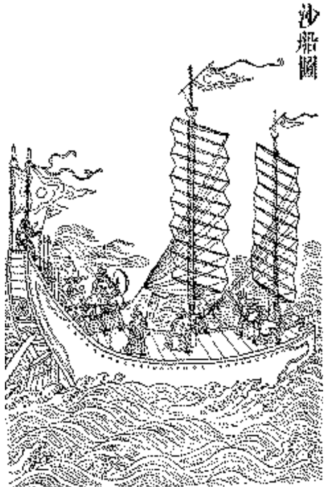
Figure 8. Illustration of fighting vessel showing axial rudder and 'steering' oar (from Audemard 1957: fig. 23)
