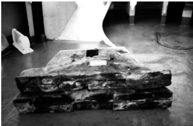
Figure 44. Shinan Ship photograph of a bulkhead/frame section from the keel area showing the waterway.
