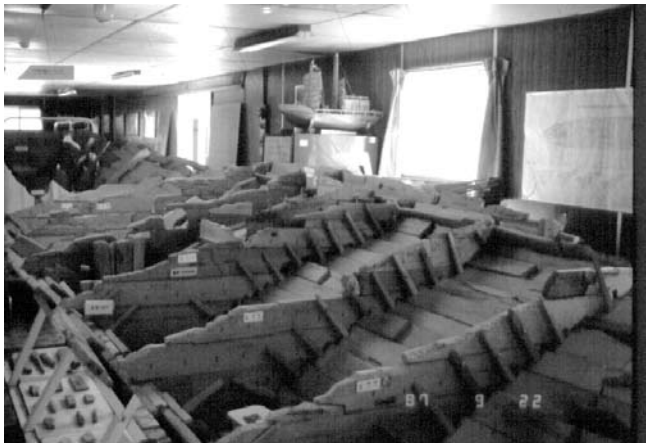
Figure 43. View of the model of the Shinan Ship showing the details of the stiffeners.
