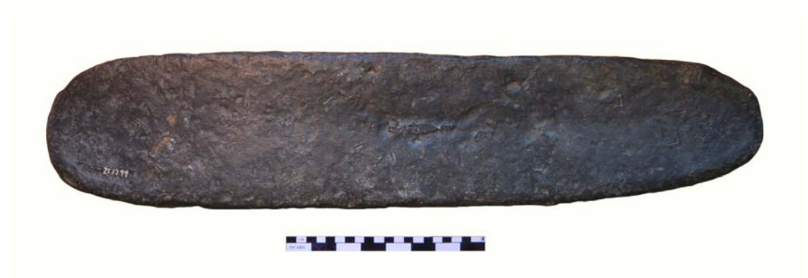
Figure 11: Cooling surface of ingot ZT 3399, Type VI. (Scale = 20 cm)
