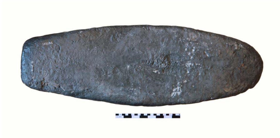
Figure 9: Cooling surface of ingot ZT 3388, Type IV. (Scale = 20 cm)
