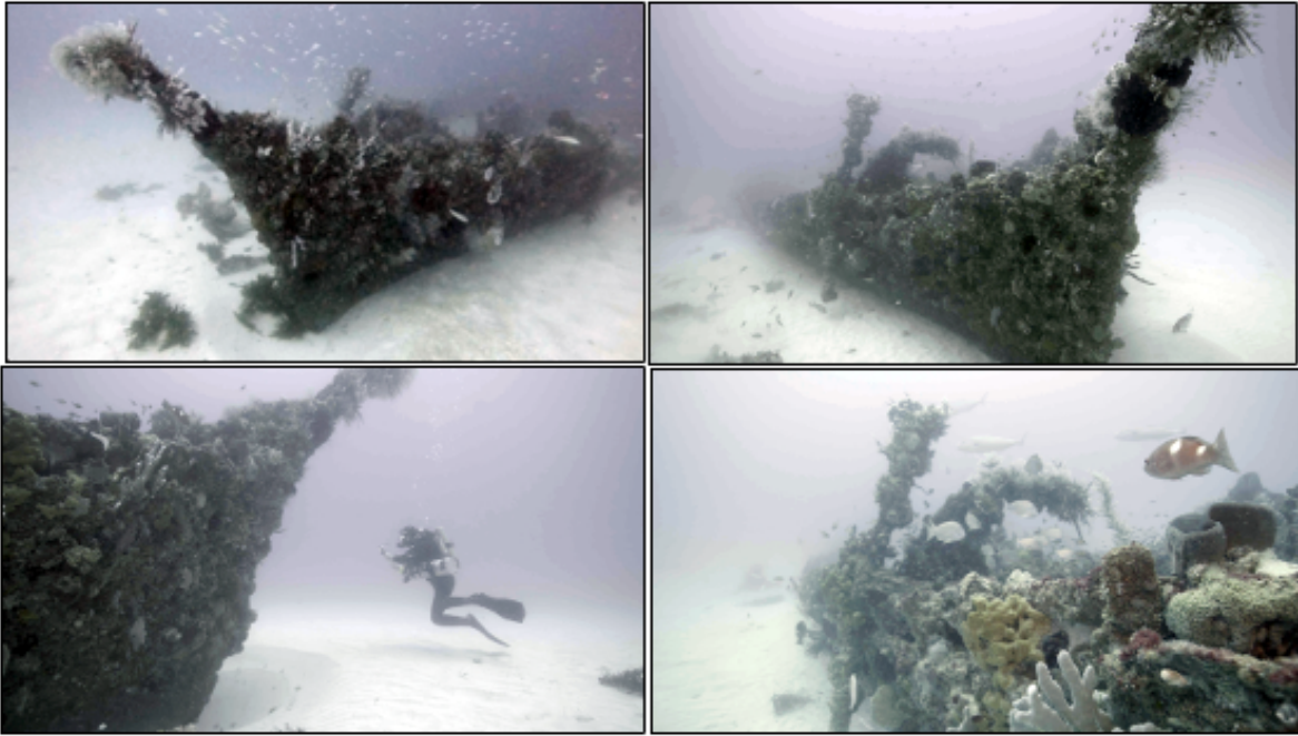
Figure 9 (Top left) Portside view of Bow. (Top right) Starboard view of bow and two anchors. (Bottom left) Diver for scale, with approximately four metres of hull protruding above seafloor. (Bottom right) two Admiralty-type anchors as seen looking down the starboard side (Images: © VAM Media).
