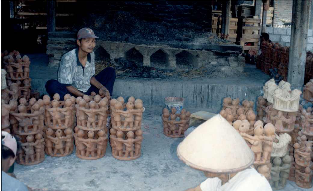
Figure 163: Worker at ‘Timboel Ceramic’ in Central Java polishing a candle-holder before glazing.
