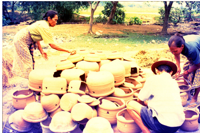
Figure 2: Women assisting man in charge of building the hipped-shaped stack of earthenware to be fired.
