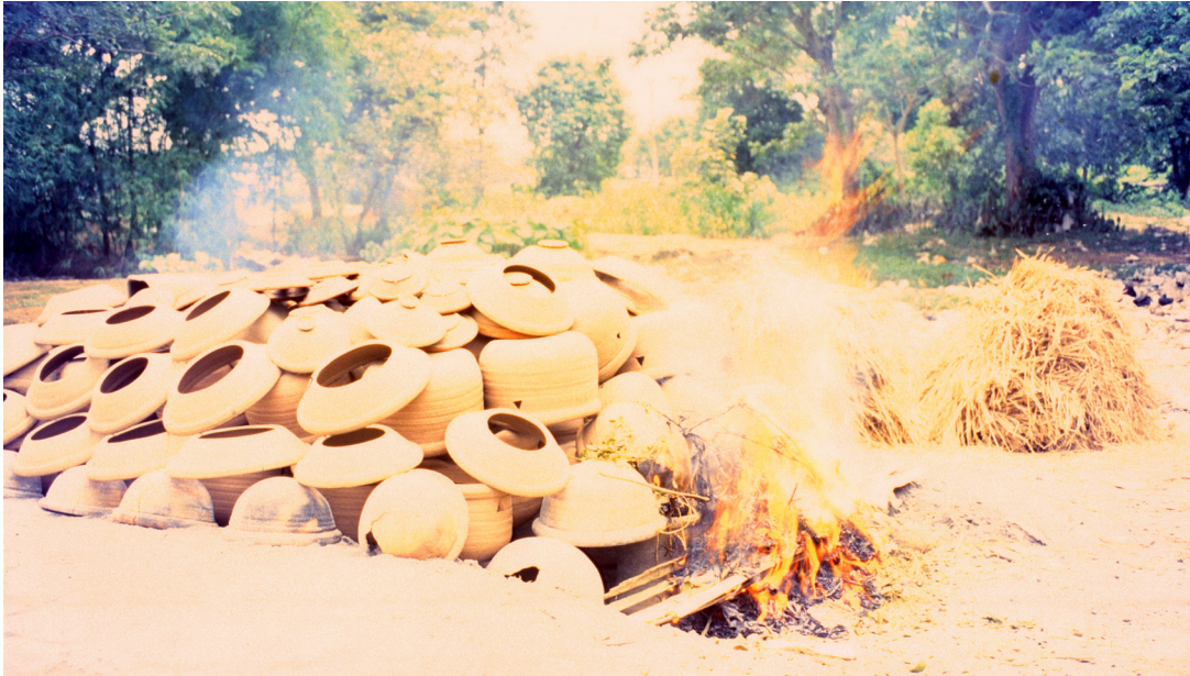
Figure 3: The fire is begun against the prevailing wind at the end of the trench. Note the large ring stands on top of the pile.
