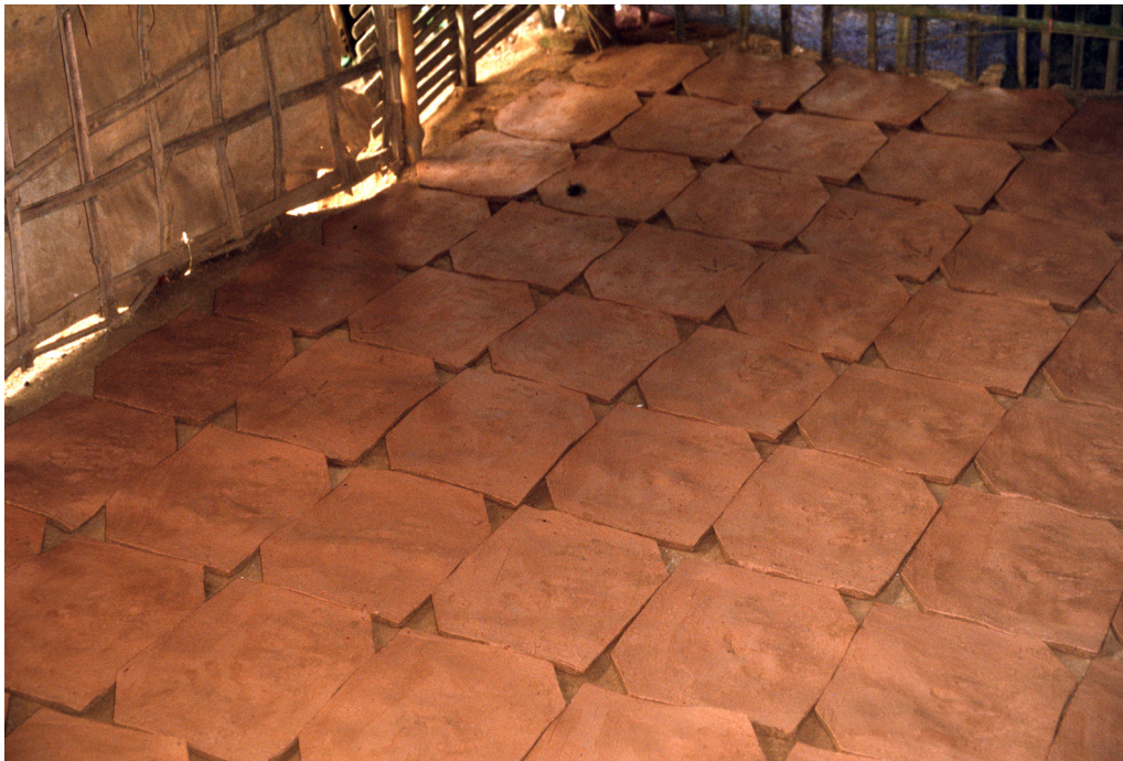
Figure 180: Drying the flat clay slabs takes place on the floor of the work shed.
