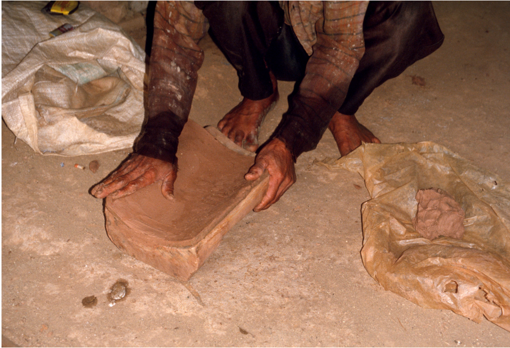
Figure 181: Shaping of the leather-hard clay slab is done in a second type of wooden mould.
