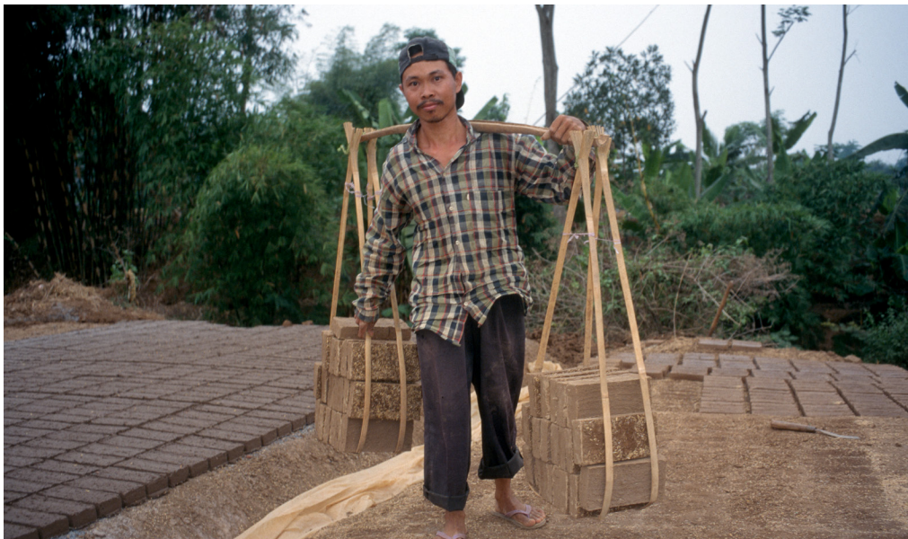
Figure 166: Worker transporting the sufficiently dried bricks to the kiln.
