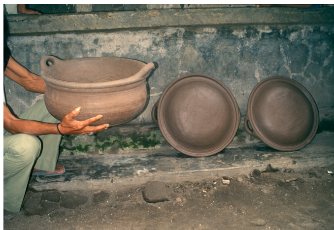
Figure 45: Parts of a cake oven, pembakaran kué , left outside a potter’s house to dry. A shrinkage of 10–15% will occur when the parts have been fired. Photographed in Bumi Jaya, Banten.
