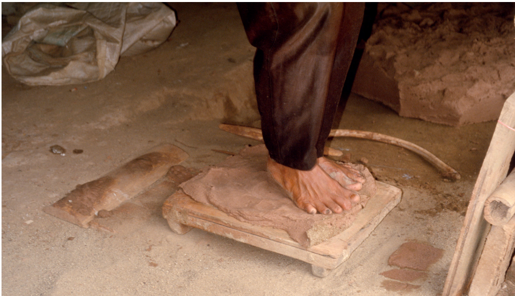
Figure 178: Pak Ajun is compacting clay in a handmade wooden roof tile mould by standing on it.
