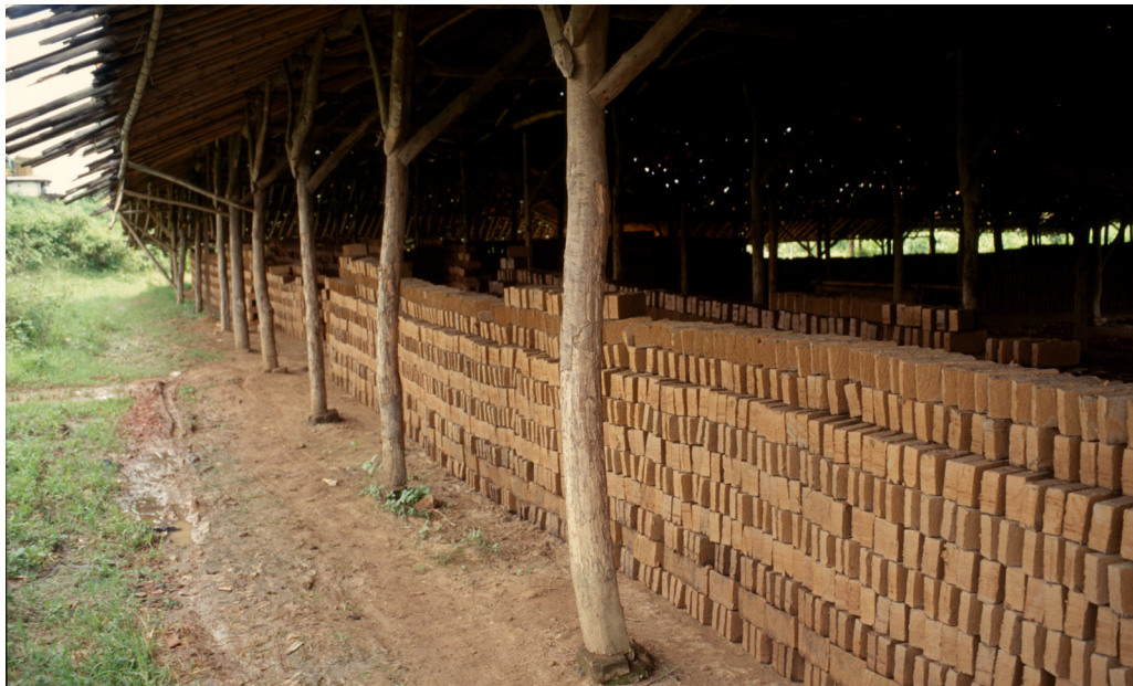
Figure 170: Bricks are stacked to dry under a thatched roof in an open-sided shed, which allows free air circulation.
