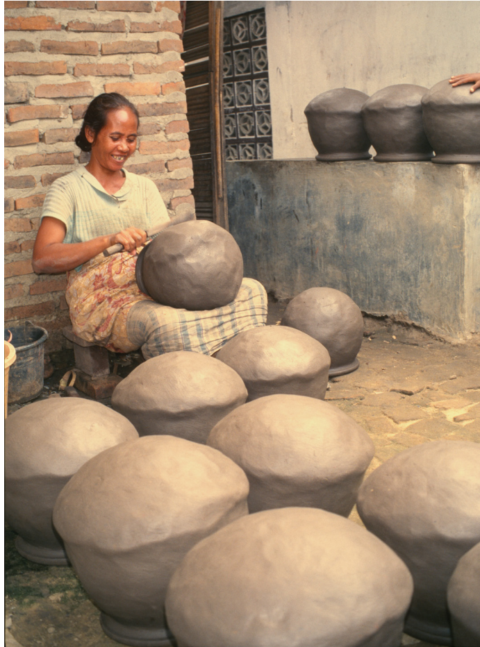
Figure 33: Potter in Bumi Jaya, Banten, using a paddle to shape a padaringan , rice jar.
