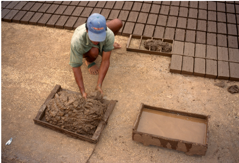
Figure 165: The brick former is dipped in water then filled with clay.
