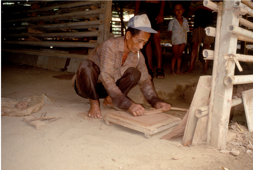
Figure 179: A wooden knife is used to smooth the clay after surplus clay has been cut off with a wire tied between both ends of a wooden bow.
