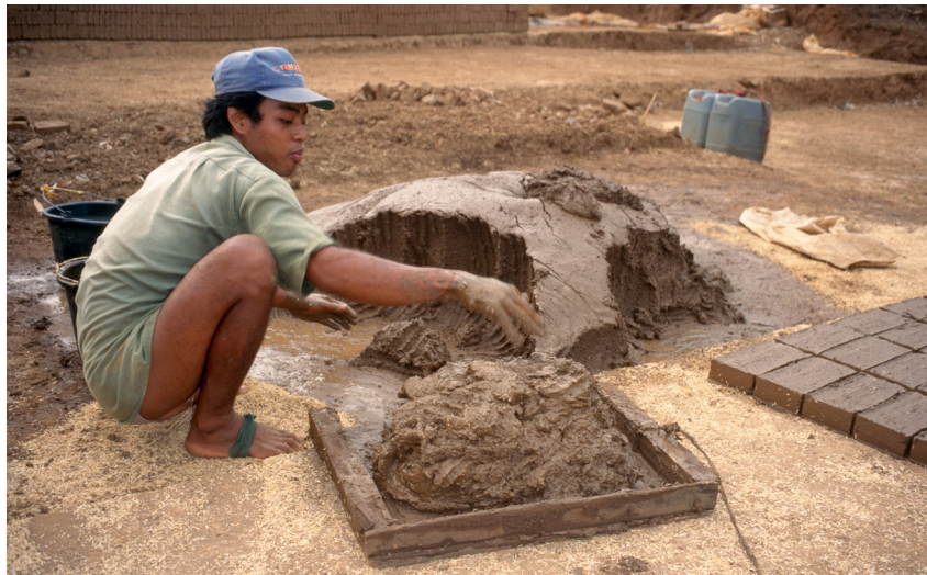
Figure 164: Noritin scoops up some of the clay from the pile of prepared brick-clay on to a tray with three sides.
