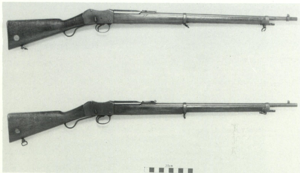
Figure 3 Martini-Enfield Rifles Mark I Modified, W.A. Pattern. The upper rifle is WA/40/D and the lower is WA/1043/D. Note the Rigby pattern nose cap/bayonet boss, which is the feature of the W.A. Pattern. The fore sight of the upper rifle has been lost and replaced by a bush blacksmith. (Photo D.Elford, W.A.M.)
