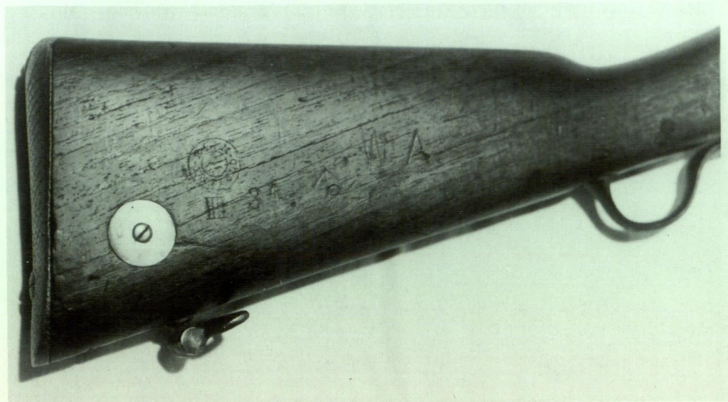
Figure 9 Butt markings of the Mark II. W.A. is punched with different, larger letter punches which have also been noted on another Mark I W.A. Pattern butt. The Enfield roundel, Mark II stamp and surplus marks are also evident. (Photo R. Stein)
