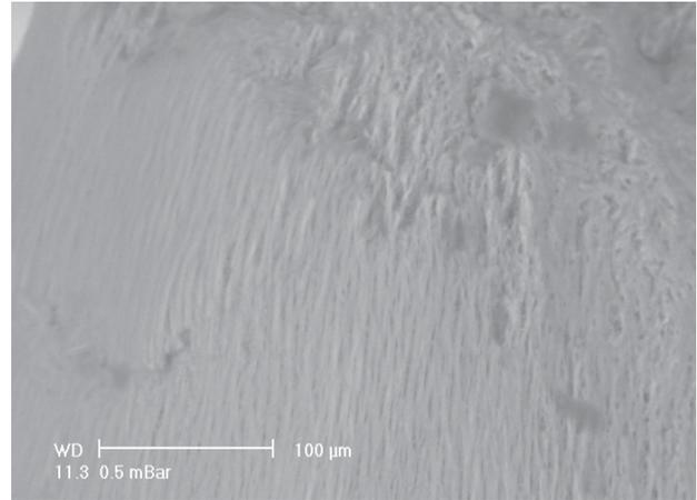
**FIGURE 7** Scanning electron micrograph of the upper section of a tooth taken from Megamouth #3 during the recent relocation, showing the damage likely to have been caused by prolonged exposure to formalin solution. Image: M. Verral.
