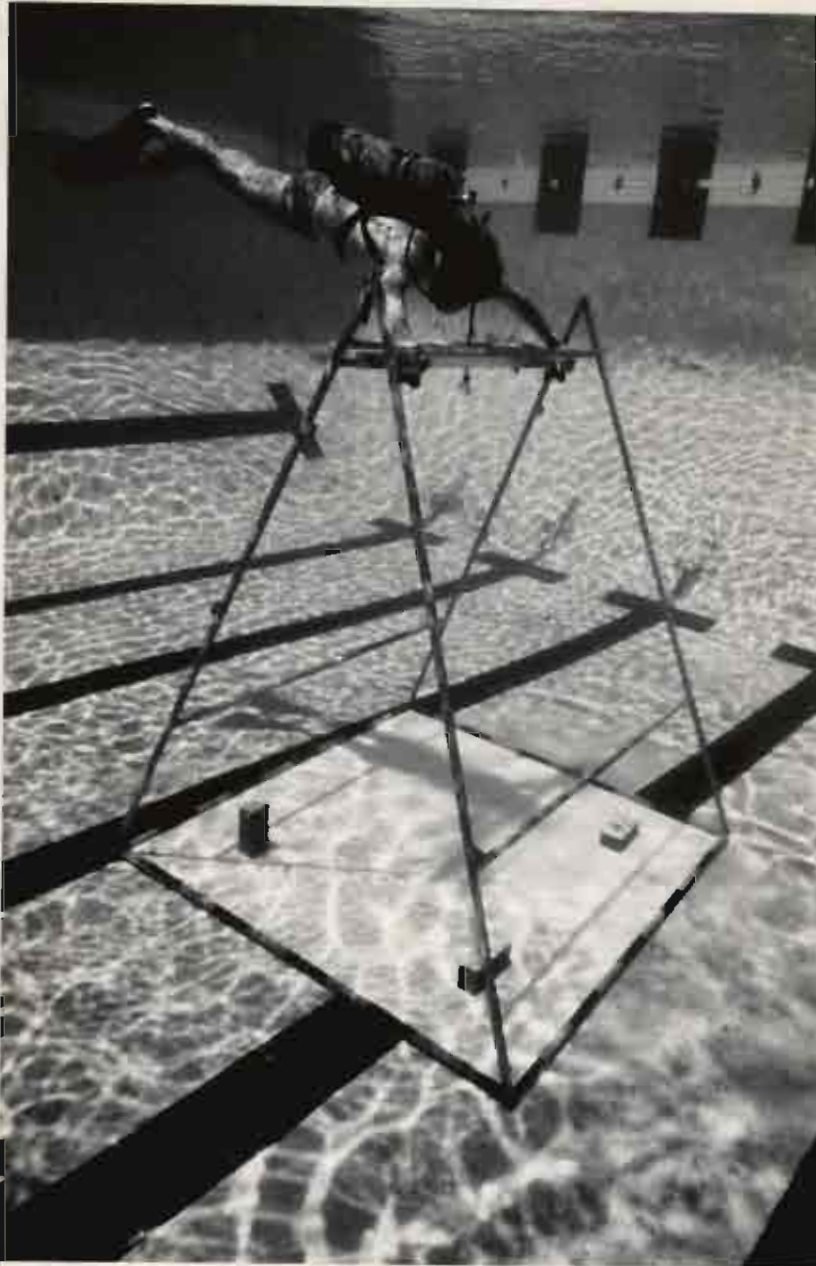
Fig. 10 Photo tower with grid square and calibrated bricks. Diver in process of taking a stereophotograph.
