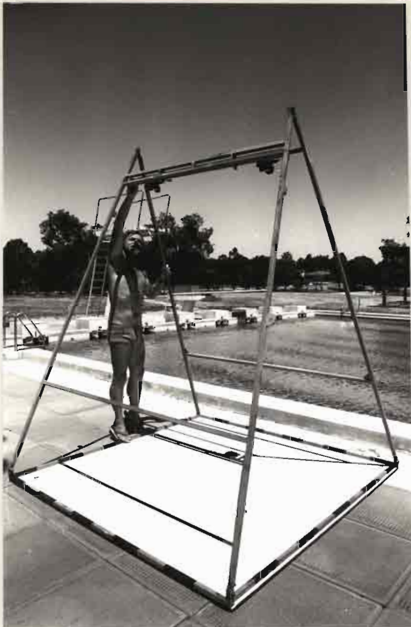
Fig. 9 Photographic tower with stereo bar in place, just prior to swimming pool trials.
