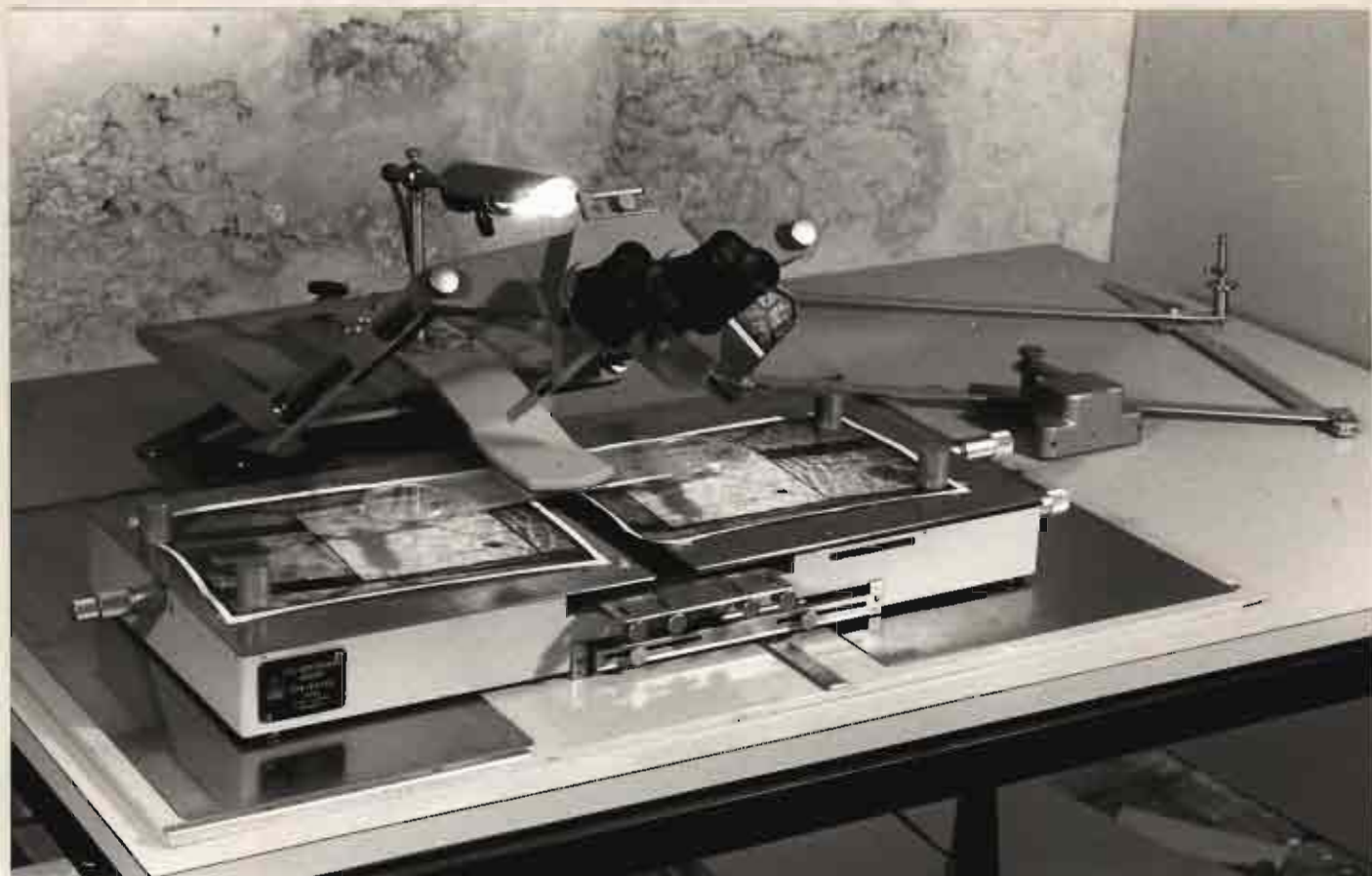
Fig. 7 Stereotope, mounted for operation.
