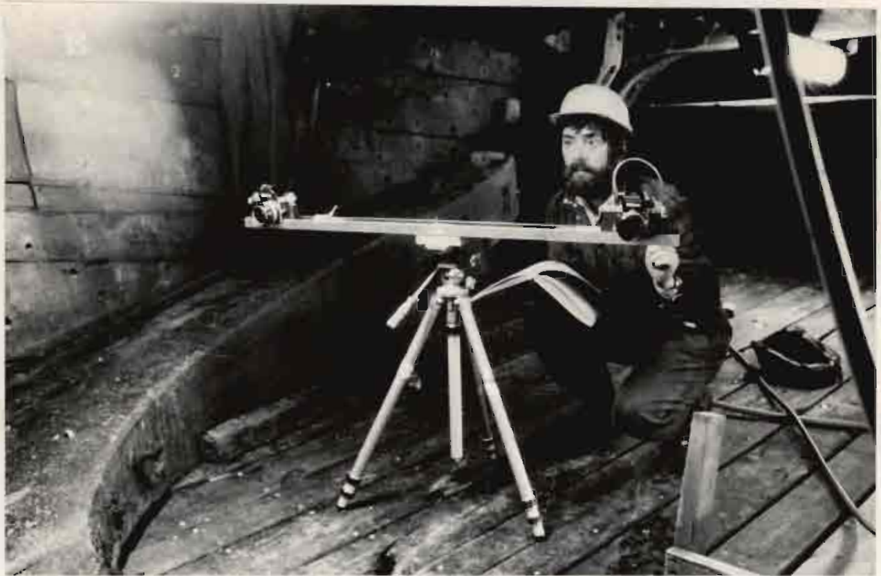
Fig. 5 Stereo recording system in use on board the Wasa .
