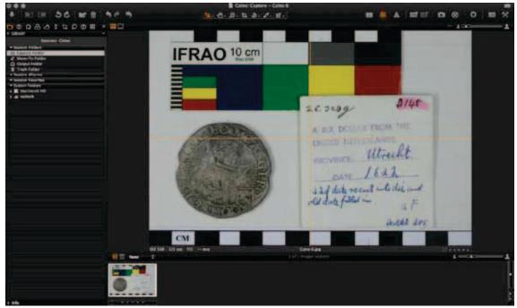
Notice both scales are in the view and that every thing is clear and in focus. If the image for some reason is washed out it may be because the camera has not been able to adjust the aperture, so manually on the camera close down the stop aperture to f32.
