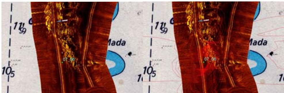
Figure 12. Side scan sonar image and magnetometer contour plot of Site 07_06. Large iron wreck near Matte Mada.
