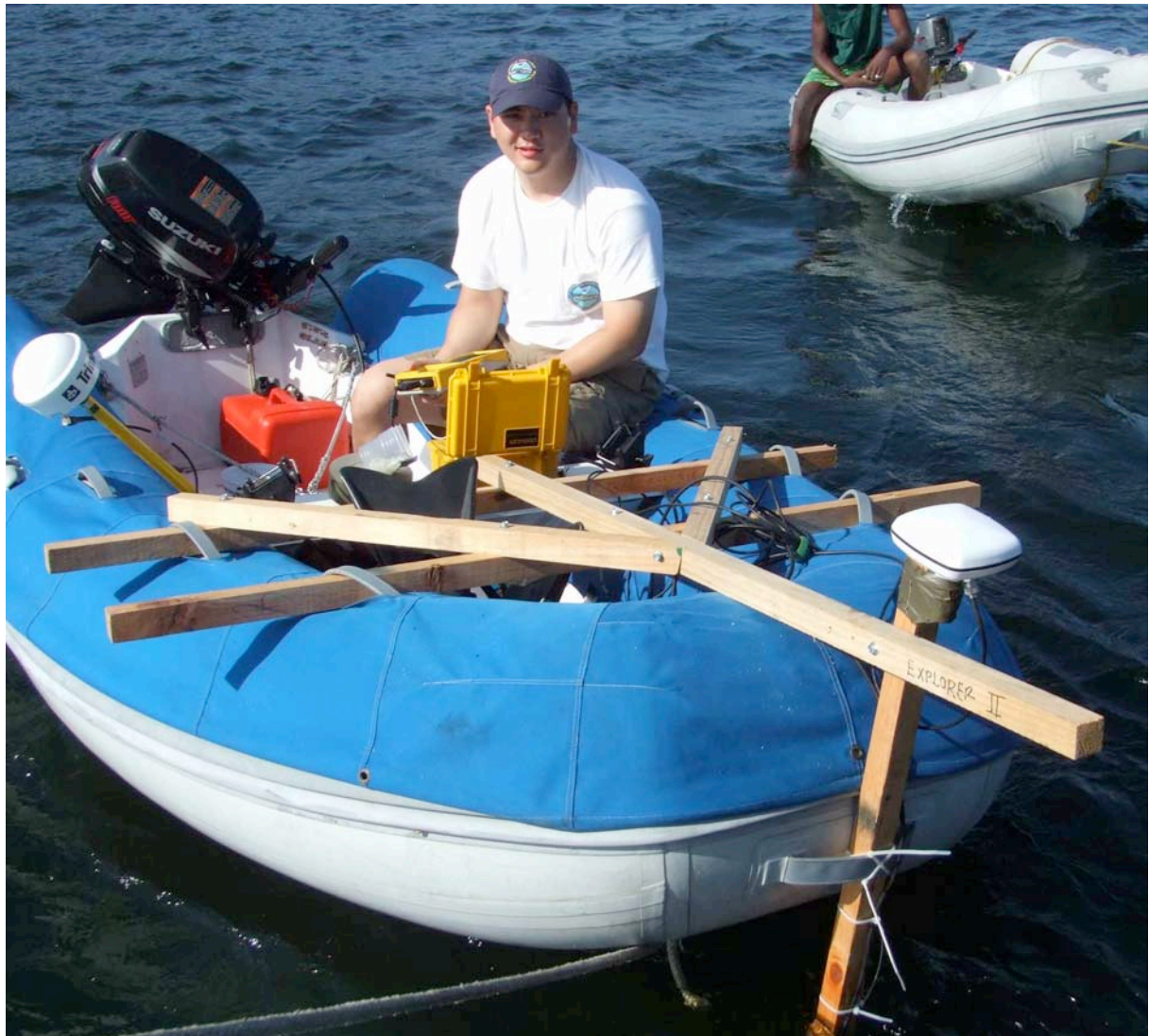
Figure 19 Oceanographer Bert Ho and the system devised to mount his sonar array to the 'rubber duck'. A useful example. M. McCarthy.
