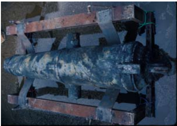
Figure 36. The James carronade after deconcretion.
