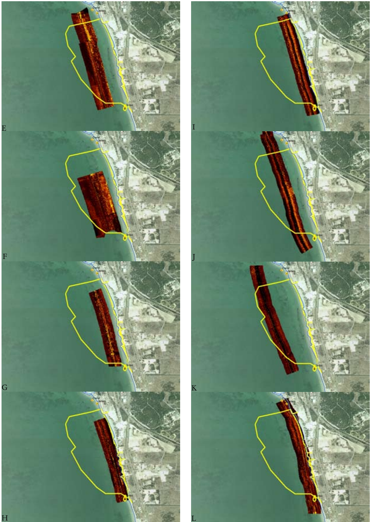
Figure 46e-l. Side scan sonar survey tracks over the Port Coogee development area.
