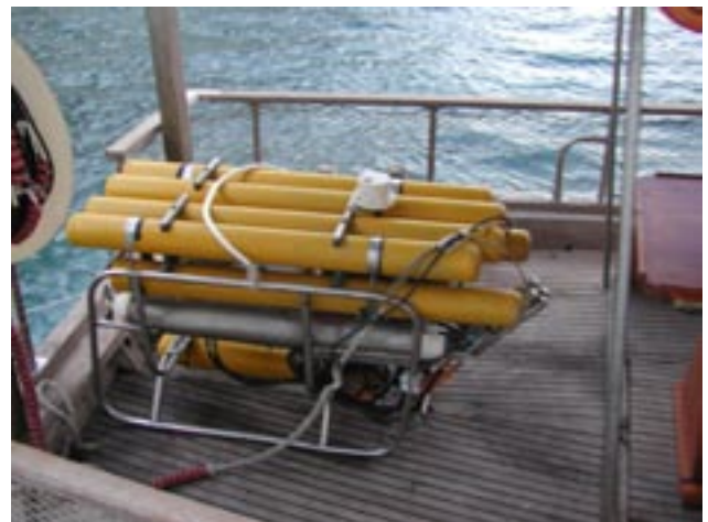
Figure 23. The ROV used to inspect the deep water sites.
